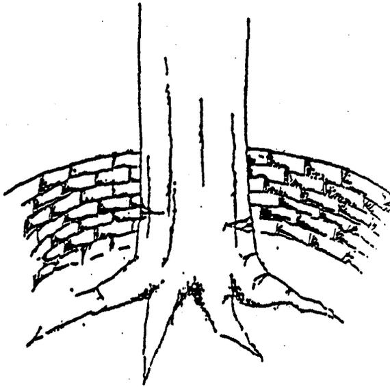
**Figure 3. Excavated root collar with retaining wall**
